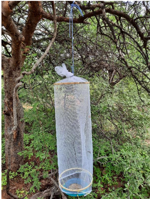
Fig. 2: Butterfly trap made of wooden embroidery hoops, hard netting, plastic plates and rope. See the documents about traps for more information.
