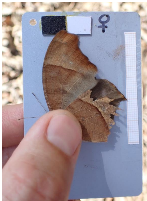
Fig. 3. Grey card with white and black standard as well as sex information. The other side of the card looks the same but has a male symbol. If the specimen has wing damage, it should be photographed from both sides. The card should be cleaned with soapy water after each day of usage. We avoid collecting data on the parts covered by the thumb.
